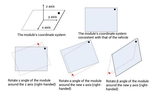
Figure 2-2 Coordinate System of the Module
