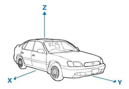
Figure 2-3 Coordinate System of the Vehicle
