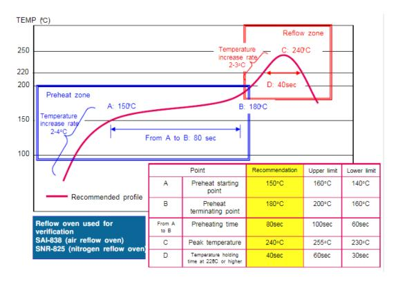
Figure 6-1 Reflow Soldering Temperature Curve
