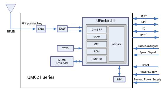
Figure 1-2 UM621 Series Modules Block Diagram
